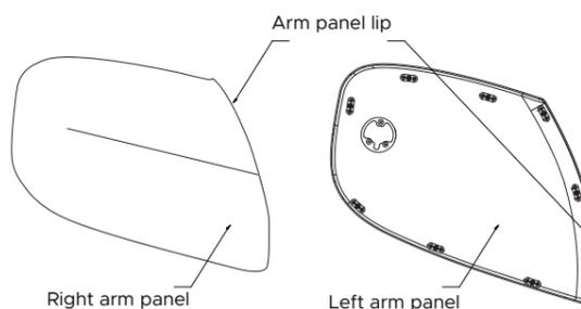
**7 STEP 7:** To attach the arm panels, align the connectors on the arm panels with the sockets on the chair body. Push firmly to connect into place.
